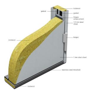
Area: External door Fire class: - El30 Smoke control: Sm/Sa Self-closing: C5 Acoustic performance: Rw 37 dB Thermal transmittance: U=1.6 W/m²·K \* Burglar resistance: RC 3 \*\* DETAILED INFORMATION Produced from galvanized steel Leaf sheet steel thickness 1,0 mm Frame sheet steel thickness 1,5 mm Door leaf thickness 62 mm
